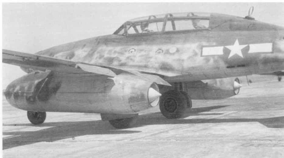
Cleaned up and bearing the US Army Air Force insignia, a two-seat Me 262B-1a trainer is flight tested in the USA. Note the extreme rear position of the second crewmember and the FuG 25a IFF radar loop antenna.
