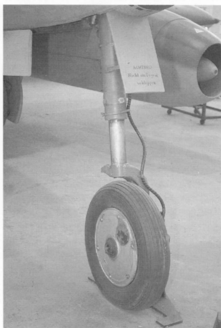
The rearward retracting nose landing gear was the crucial last shift in major design features in a sequence of several modifications that included a fully swept wing leading edge and more effective horizontal stabilizer trim.
