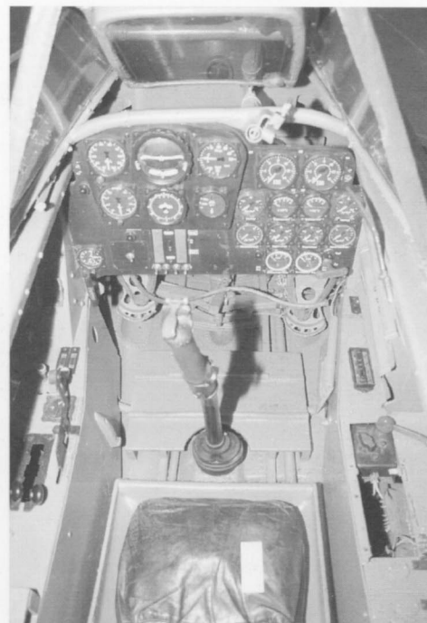
The instrument panel layout has the standard flight instruments on the left and the all-important engine gauges on the right. Throttles and engine start were on the left hand console but required two hands and sloppy co-ordination could lead to flameouts or stalling. The consequences of this were to render the engine inoperable until it cooled.
