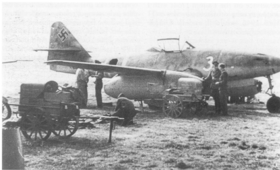
Field servicing trolleys stand by this Me 262. For all its radical concept, the fighter was relatively easy to maintain and put in the air. Messerschmitt paid particular attention from the outset to production and in-service maintenance needs.
