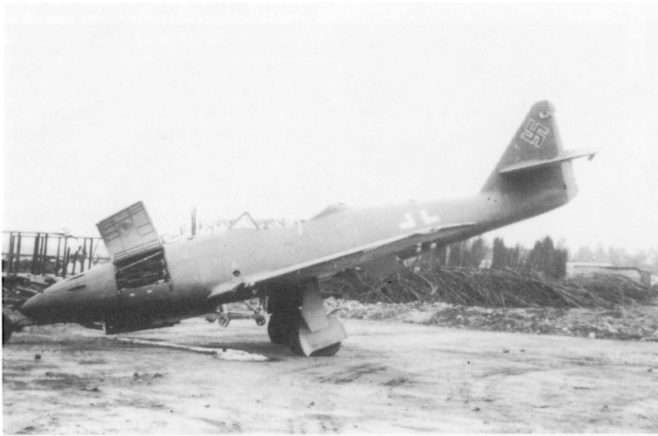
Stripped of engines and nose leg, this Me 262 had a final resting place in the scrapyard. Note the generous access door in the forward fuselage aft of the four cannon ports.
