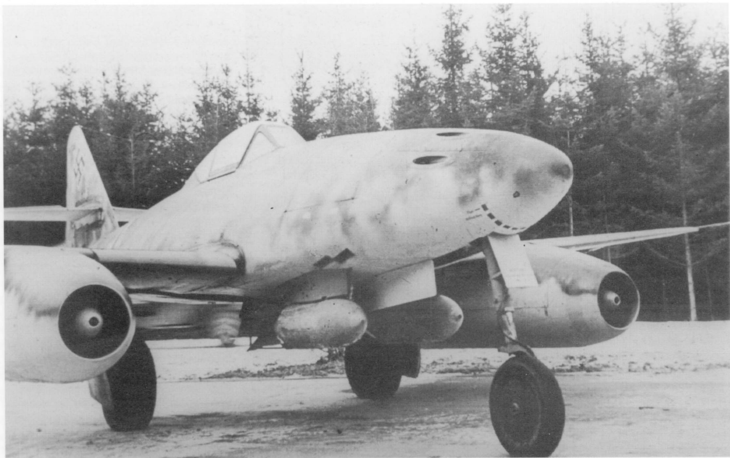
A fine shot of Me 262A-1a werke/nr 110813 deployed initially with III/EJG 2 and then with KG(J) 51. Note the spent cannon shell ejector 'chutes immediately above the bomb pylon and the gun camera port in the extreme nose.
