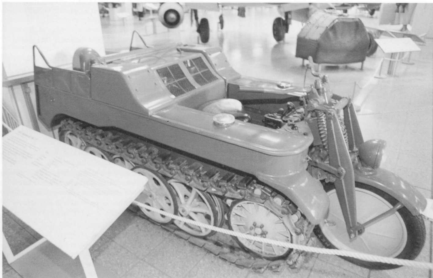
Beautifully preserved in the Deutsches Museum, a Kettenkrad tractor used at Me 262 airfields for moving the aircraft around. With extraordinary pulling power for its size, the tracked vehicle was adapted for many informal uses and on one occasion during an air raid doubled as an open top ambulance when collecting an injured Adolf Galland from his crashed aircraft.
