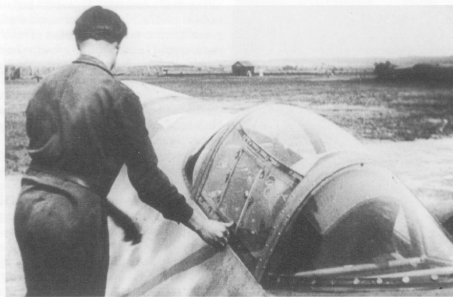
The early design of canopy and frame arrangement incorporated considerable ironwork and is a far cry from the full blown canopies of the 1990s. Note the small side hatch on the port side between vertical frames. The cockpit configuration was designed to support an ejection seat.
