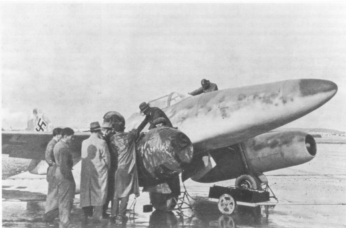
Looking uncharacteristically tail-heavy, the third Me 262 prototype (PC+UC) was the first to fly with all-jet propulsion, one of four aircraft to have a tail-wheel.
