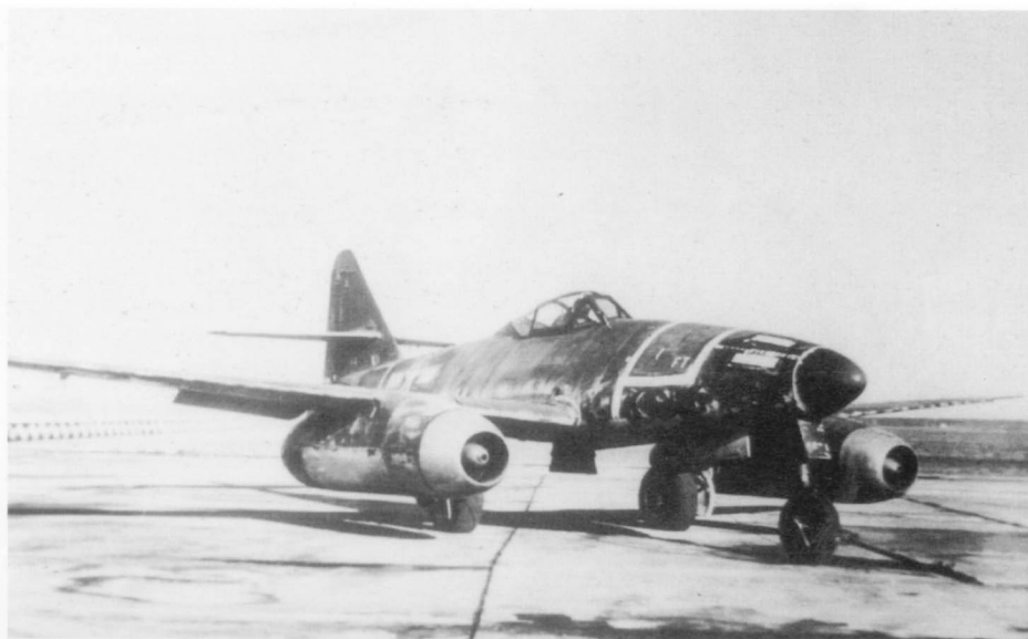
For those aircraft that managed to survive the rigours of the war's end, exterior skins were frequently a mix of original and replacement panels. Note the changes in colour on this captured aircraft around the forward fuselage and forward nacelle sections, indicative of changeouts.
