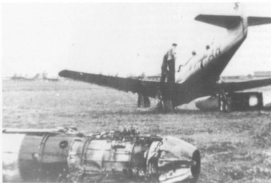
Nose gear failures were not uncommon and, due to engineering layout, frequently led to serious damage. In this incident an early pre-production aircraft has lost both engines after nosing into soft ground.
