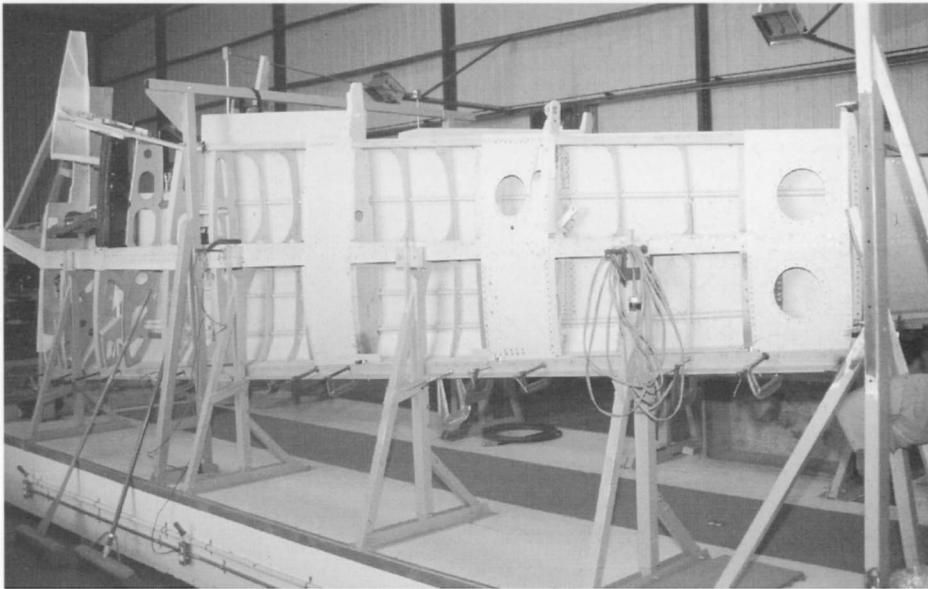
Seen in its jig, the right hand wing of one of the replicas shows Tischler's superb workmanship and attention to detail.
