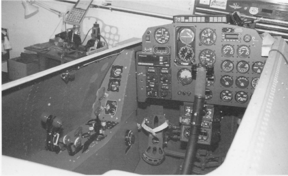
Fine workmanship with craftsmanship and care denied to most of the hurriedly produced originals define the replicas Herb Tischler builds. Here an almost completed cockpit shows the original instrumentation and the almost obligatory modern radios needed to fly in today's crowded airspace.
