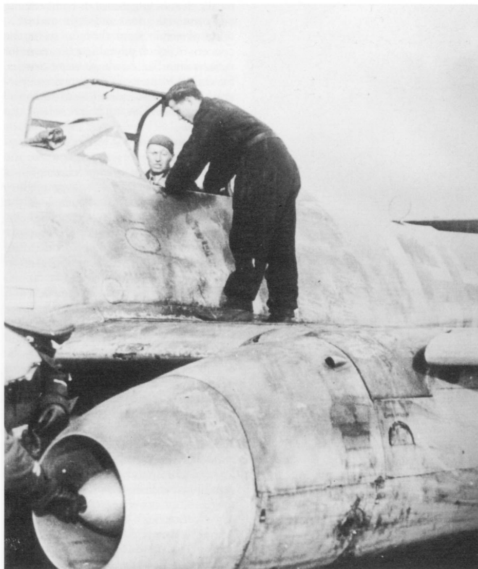
A potential source of problems with an already troublesome engine design, the Reidel starter motor housing, is clearly seen in the intake nozzle of the Jumo 004 engine nacelle. Also visible are the conveniently placed footholds for access to the top of the wing and the leading edge slat.
