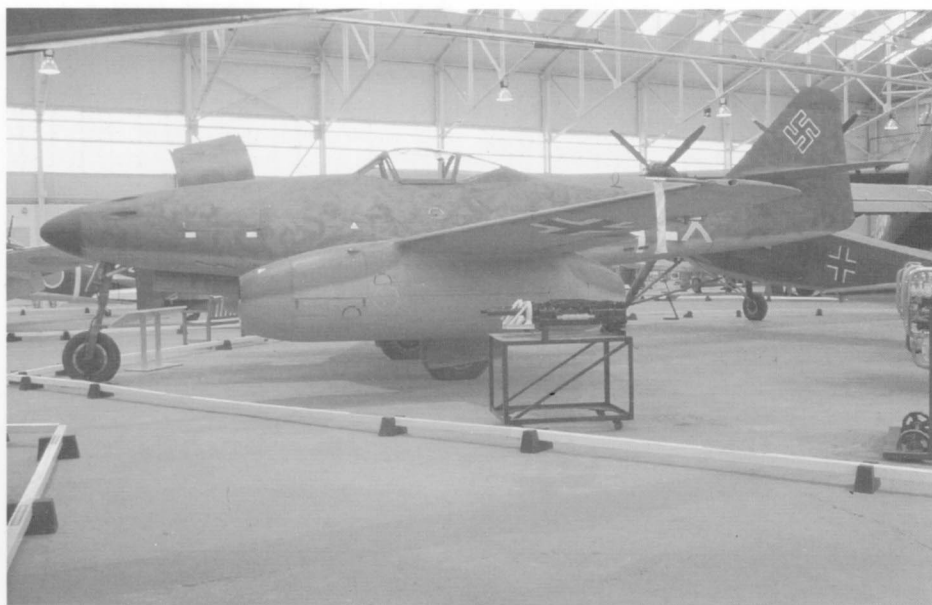
Born through expediency when engineers could not guarantee that the jet engine's girth would remain inside tolerances for a wing mounting, the underslung nacelle began a trend that would be adopted after the war.
