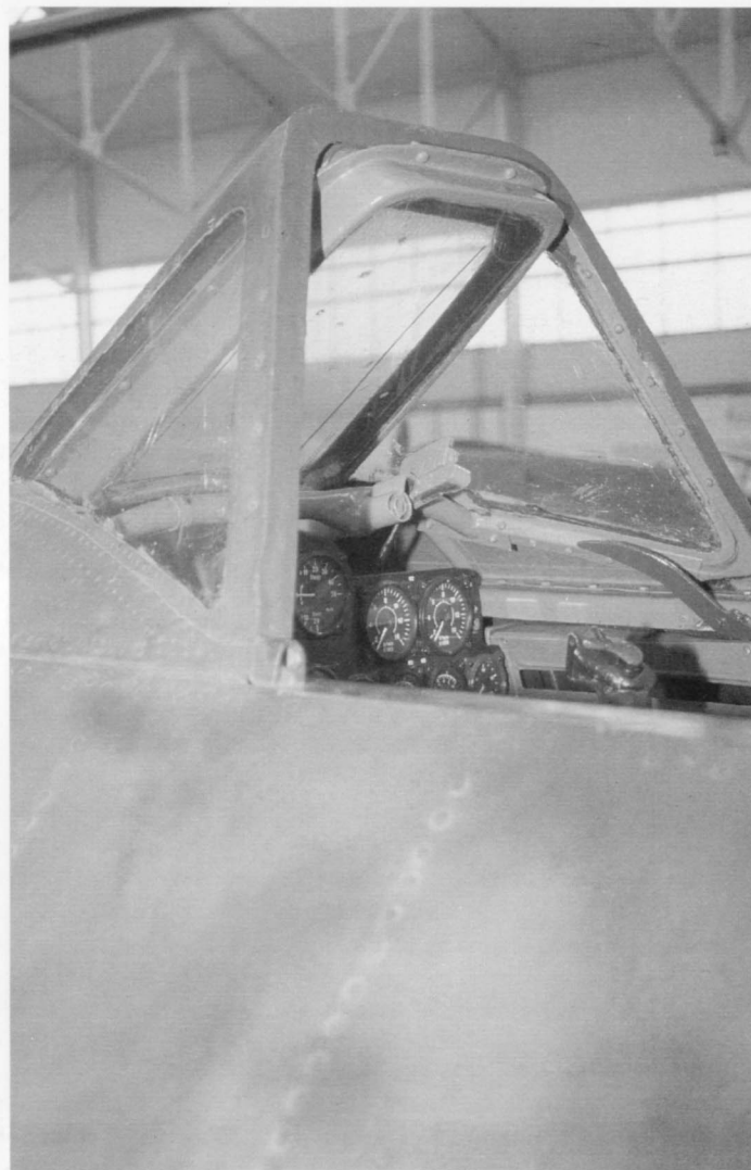
(Left) The production canopy was a sideways opening perspex bubble that gave good all round visibility and was a great improvement on earlier types such as the Bf 109.
