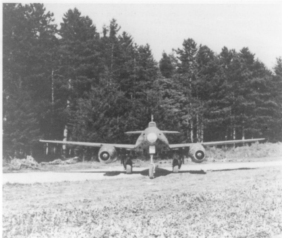
The relatively small frontal area made the Me 262 difficult to see in a head-on attack, but without a propeller in front the pilot had an excellent field of view.
