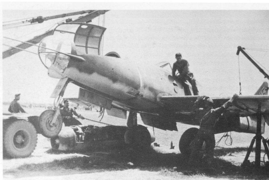
A second Me 262A-2a/U2, werke/nr 110555, was adapted as a fast two-man bomber. The second crewmember was to have lain prone and used a Lofte 7H bomb sight.
