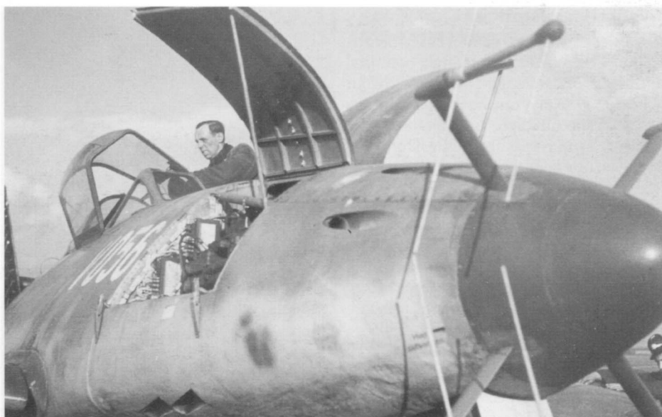
The prototype Me 262B-2a night fighter version reveals the copious cannon access bay, gun ports and ejector chutes. The generous access afforded equipment located in the nose was welcomed by ground crew used to the cramped forward fuselage of the conventional, piston engined, fighter.
