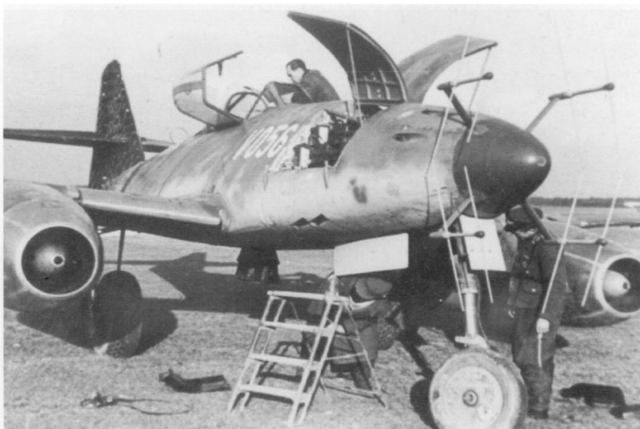
Prototype veteran V056 provided flight test engineers with a wealth of aerodynamic and directional stability information before it was adopted as the workhorse for tests of the two-seat night fighter version equipped with radar.
