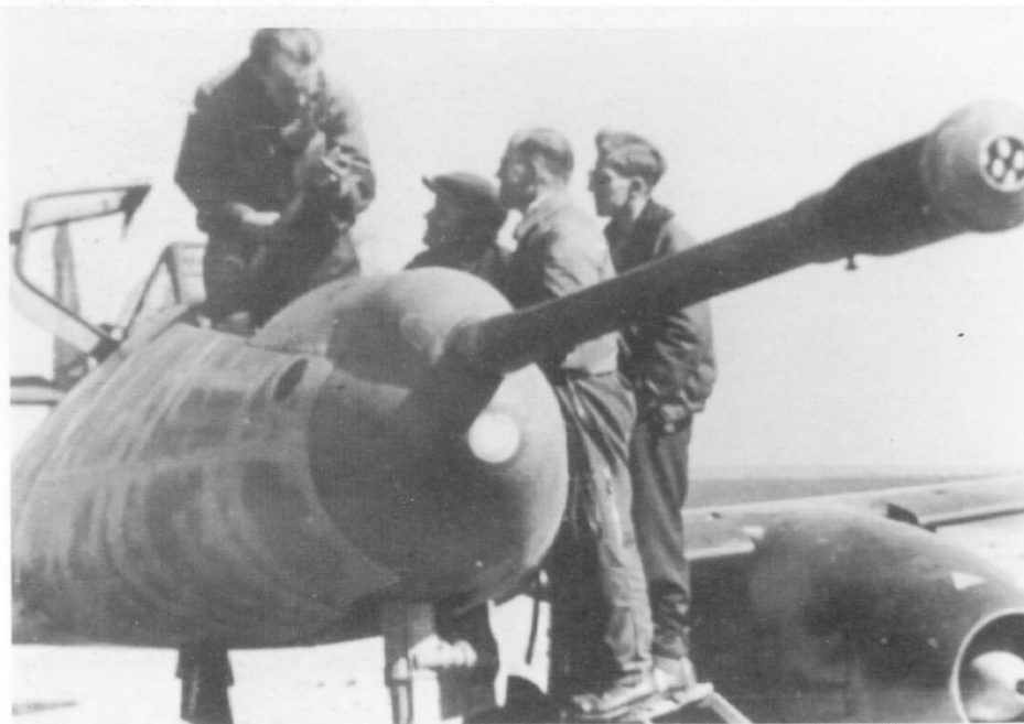
The massive 50mm MK 214A cannon replaced the four 30mm MK 108 cannon usually fitted to the forward fuselage. The MK 214A gave trouble during flight tests and frequently jammed. Note the bulbous fairing which distorts the clean lines of the fuselage nose.
