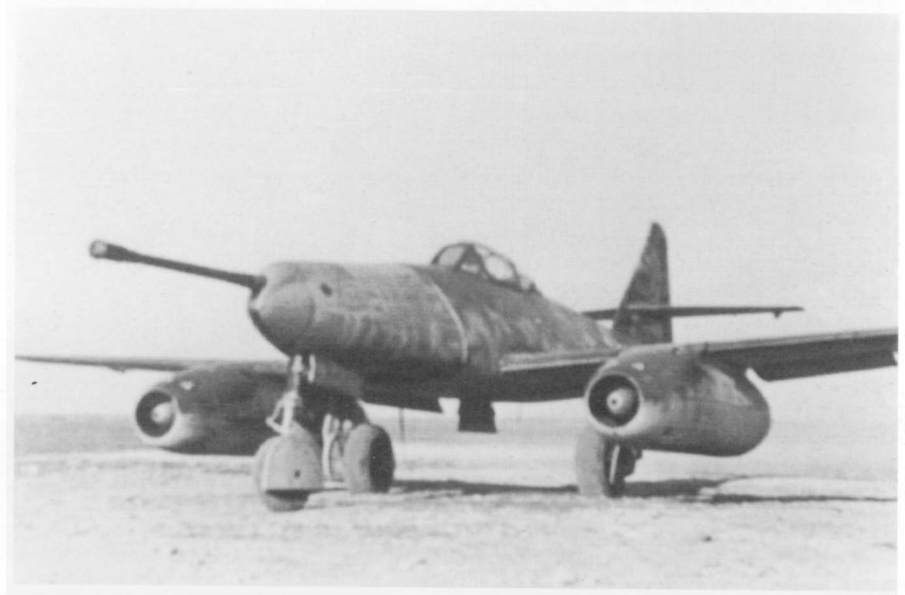
Me 262A-1a/U4 with its 50mm cannon makes an impressive picture but gave little hope for success in trials that were to reveal serious deficiencies with the concept. Although displaying a high muzzle velocity, the gun was difficult to use, unreliable and degraded the primary advantage of the Me 262 – speed. The concept was not liked by Galland and other top scoring aces, who preferred a multi-cannon arrangement blended into a streamlined shape to optimise combat capability.
