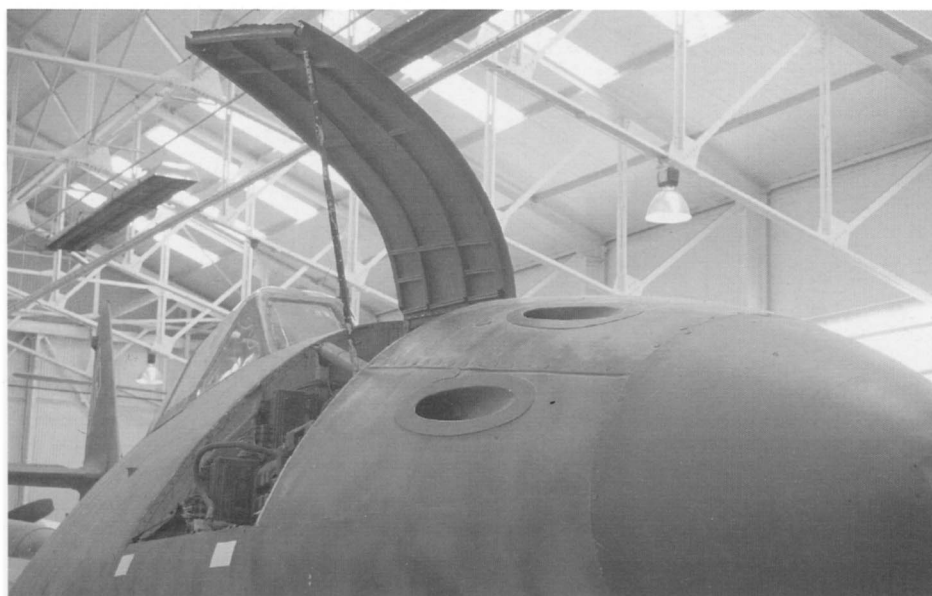
Access to the cannon was from a large panel either side of the nose giving plenty of room for the armourers.
