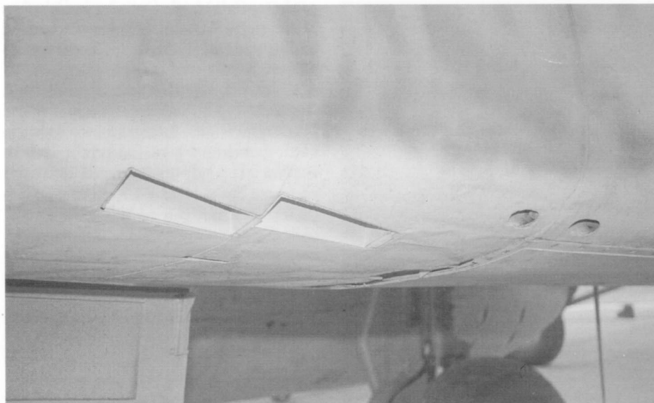
Spent ammunition cartridges were ejected downwards either side of the nose wheel bay.
