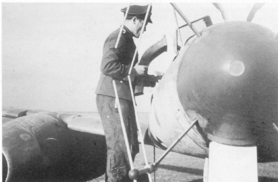
Holding a spent cartridge ejector chute, an armorer services the weapons bay on V056. The blanked-off gun camera port is clearly visible in the extreme nose.
