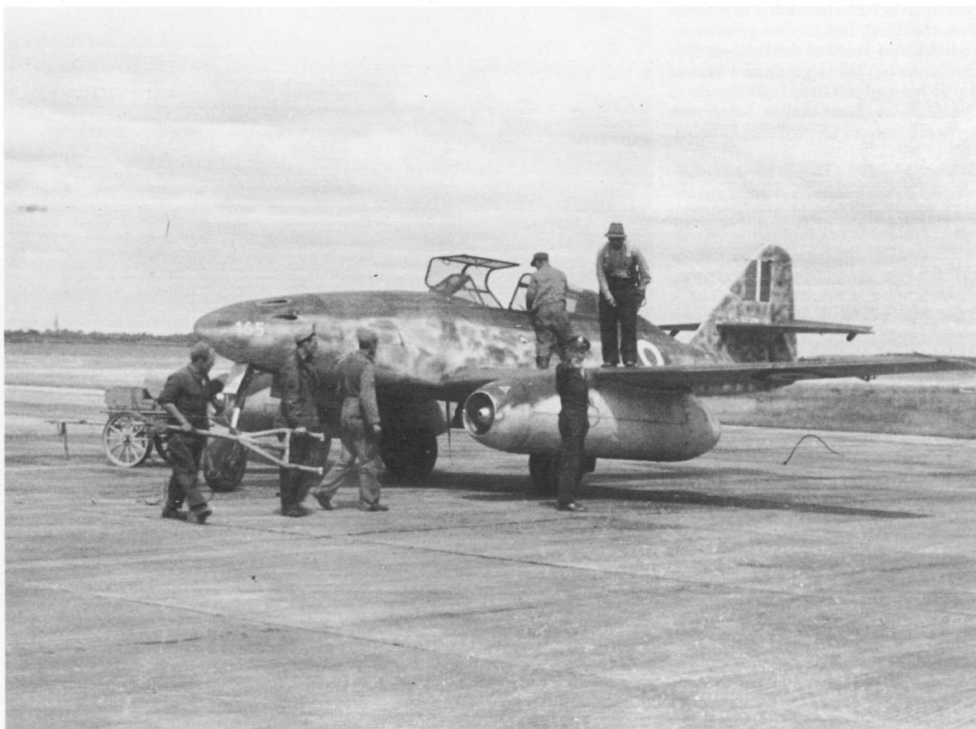
A captured two-seat Me 262 repainted with RAF insignia over standard late-war camouflage. Note the forward landing gear yoke and tow bar.
