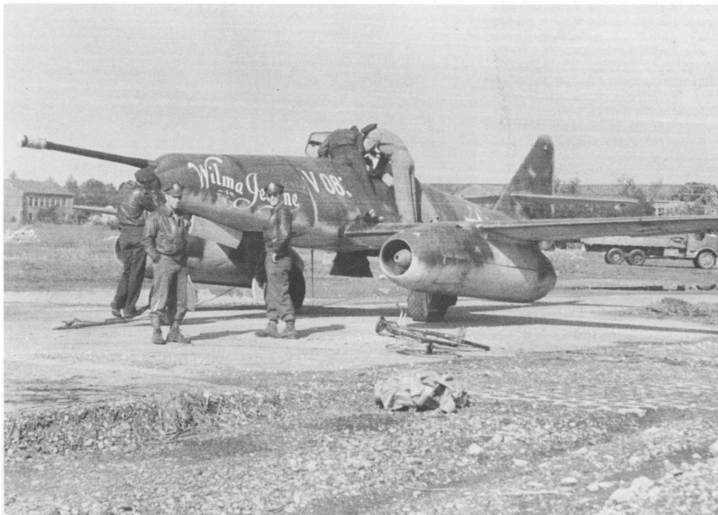
One of two aircraft modified to take the 50mm cannon, aircraft 170083 is seen here after capture by the Americans. Note the removal of the swastika and the application of the 'stars and bars' to the fuselage and (unseen) appropriate wing surfaces as per US regulations.
