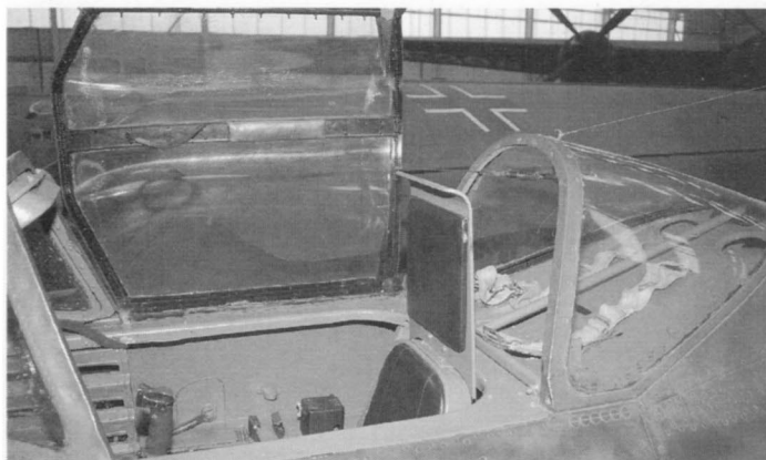
(Left) The production canopy was a sideways opening perspex bubble that gave good all round visibility and was a great improvement on earlier types such as the Bf 109.
