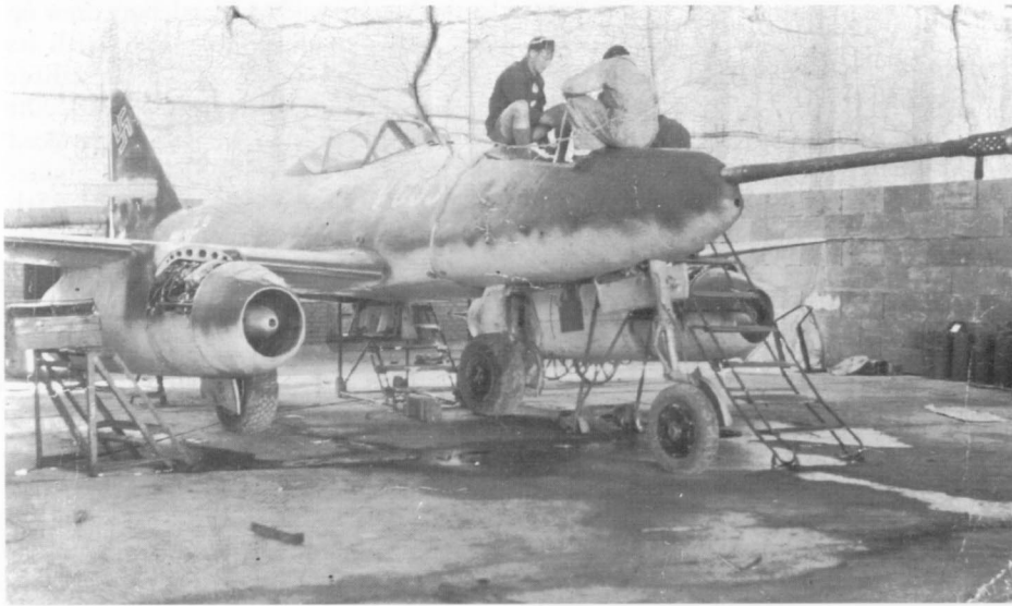
Fitted with a 50mm Rheinmetall-Mauser MK 214A cannon, Me 262A-1a/U4 ( werke/nr 111899) is seen in the checkout bay prior to in-flight firing tests. Tests were also conducted with Me 262A-1a werke/nr 170083.
