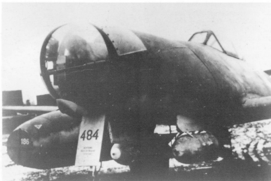
Carrying a second crewmember in a modified airframe, Me 262A-2a/U2 werke/nr 110484 was tested by Bauer and Lindner as a two-man bomber. Armament was removed and the metal nose section was replaced by a wooden section, but the aircraft came too late to offer advantages when fighters became top priority.
