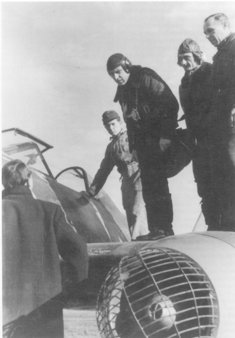
Protected from ingestion damage by a wire screen over the Jumo 004 intake, the engines on this Me 262 are about to be started as the pilot discusses final checks with Curt Zeiller.
