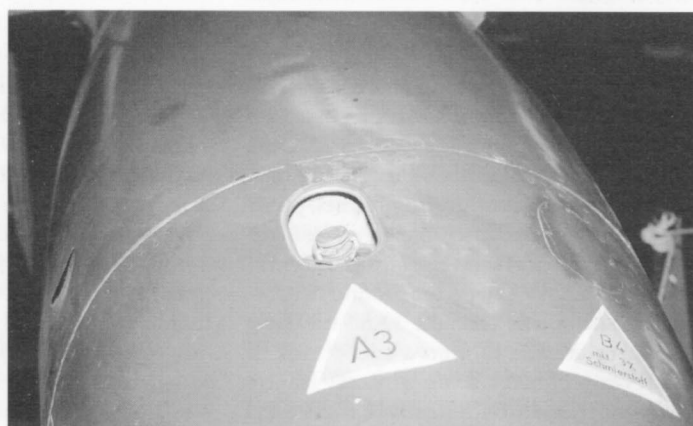
Fuel and oil for the two-stroke starter motor was contained in small tanks in the forward part of the nacelle, above the engine.
