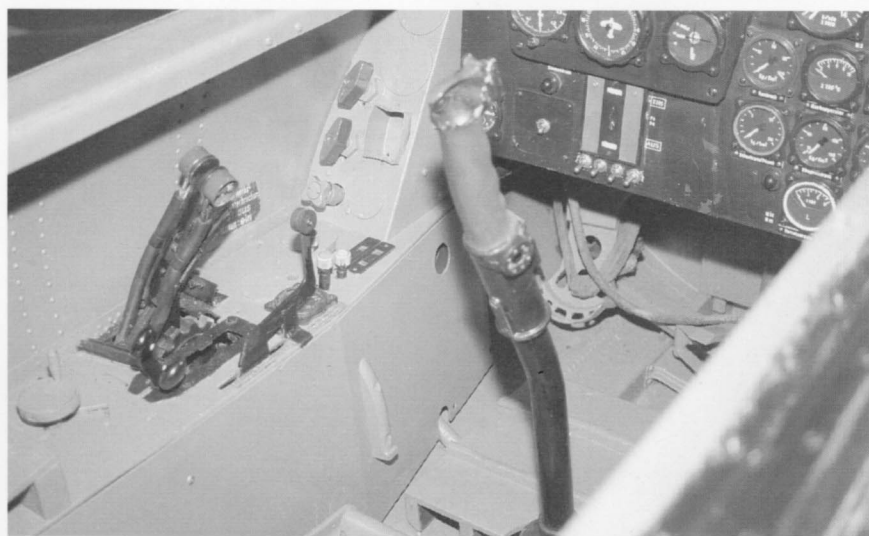
The instrument panel layout has the standard flight instruments on the left and the all-important engine gauges on the right. Throttles and engine start were on the left hand console but required two hands and sloppy co-ordination could lead to flameouts or stalling. The consequences of this were to render the engine inoperable until it cooled.
