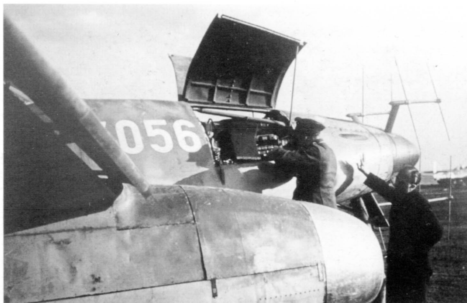
Battered engine panels and crumpled forward fuselage skins testify to the extensive use of V056 on numerous test flights. Note the leading edge slats.
