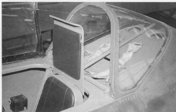
(Below) In common with other Luftwaffe types, the Me 262 had an armour plate protecting the back of the pilot's head which also acted as a headrest.
