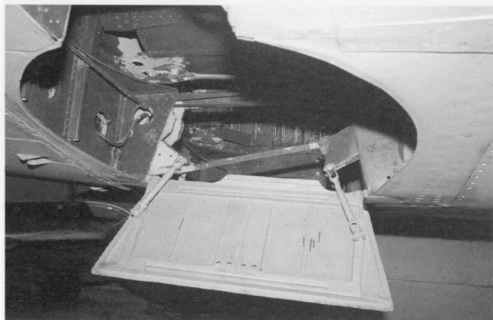
(Right and below) The robust main gear retracted inwards, rather than outwards as on the Bf 109, giving a wider track and greater stability on the ground. Once retracted, the wheels lay under the pilot's seat and the wells were covered by small doors.
