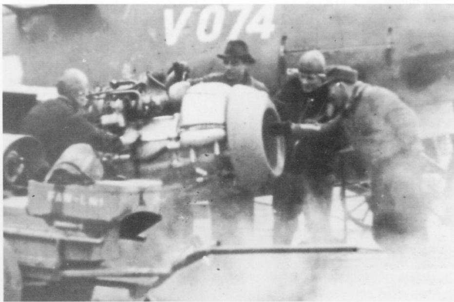
Prototype V074 was used for tests with the BMW 003A-1 jet engine incorporating a BMW 109-718 liquid fuel rocket motor. The hybrid engine combination was to have powered the Me 262C-1b, or Heimatschutze II , interceptor.
