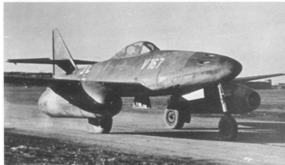
Designated as the replacement V5 prototype when the first was written off in February 1944, V 167 made more than 300 flights on stability tests and the aircraft was eventually used for trials with a new landing gear yoke.
