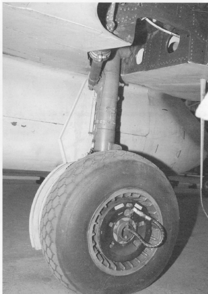
(Right and below) The robust main gear retracted inwards, rather than outwards as on the Bf 109, giving a wider track and greater stability on the ground. Once retracted, the wheels lay under the pilot's seat and the wells were covered by small doors.
