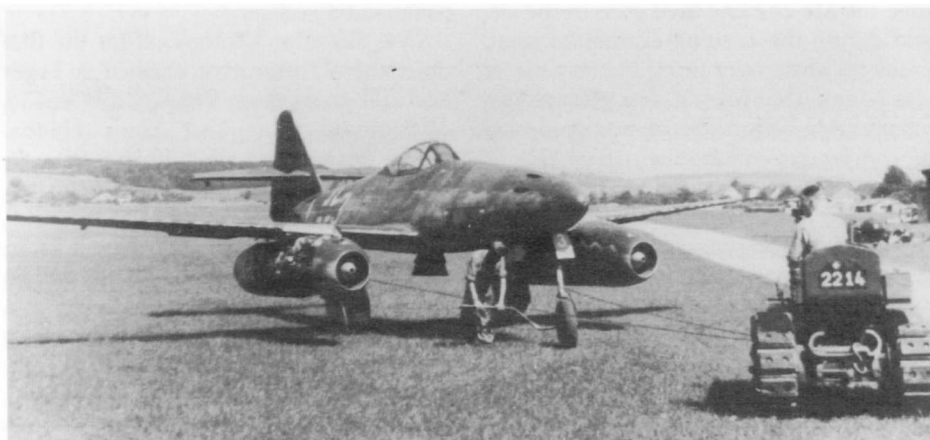
Cables attached to the main landing gear legs connect this Me 262 to the Kettentraktor tractor while a ground crewman turns and locks the nose leg before attaching a tow boom.
