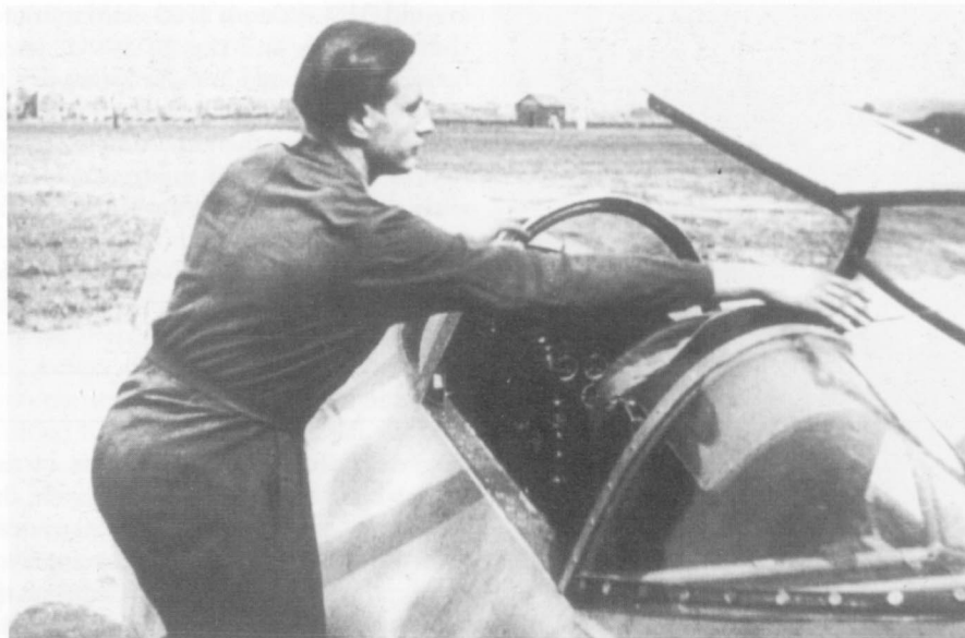
The early design of canopy and frame arrangement incorporated considerable ironwork and is a far cry from the full blown canopies of the 1990s. Note the small side hatch on the port side between vertical frames. The cockpit configuration was designed to support an ejection seat.
