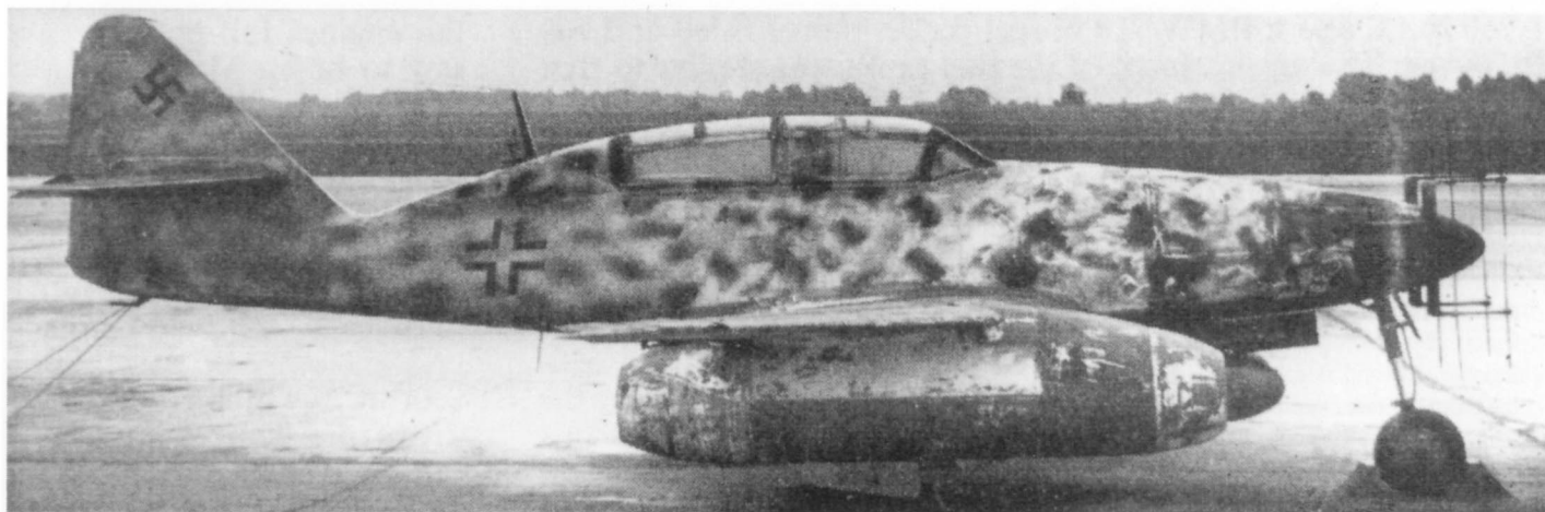
Adaptation of the single-seat Me 262 fighter into two-seat trainer and night-fighter versions necessitated the addition of a second seat in the forward section of the rear fuselage, as seen here.
