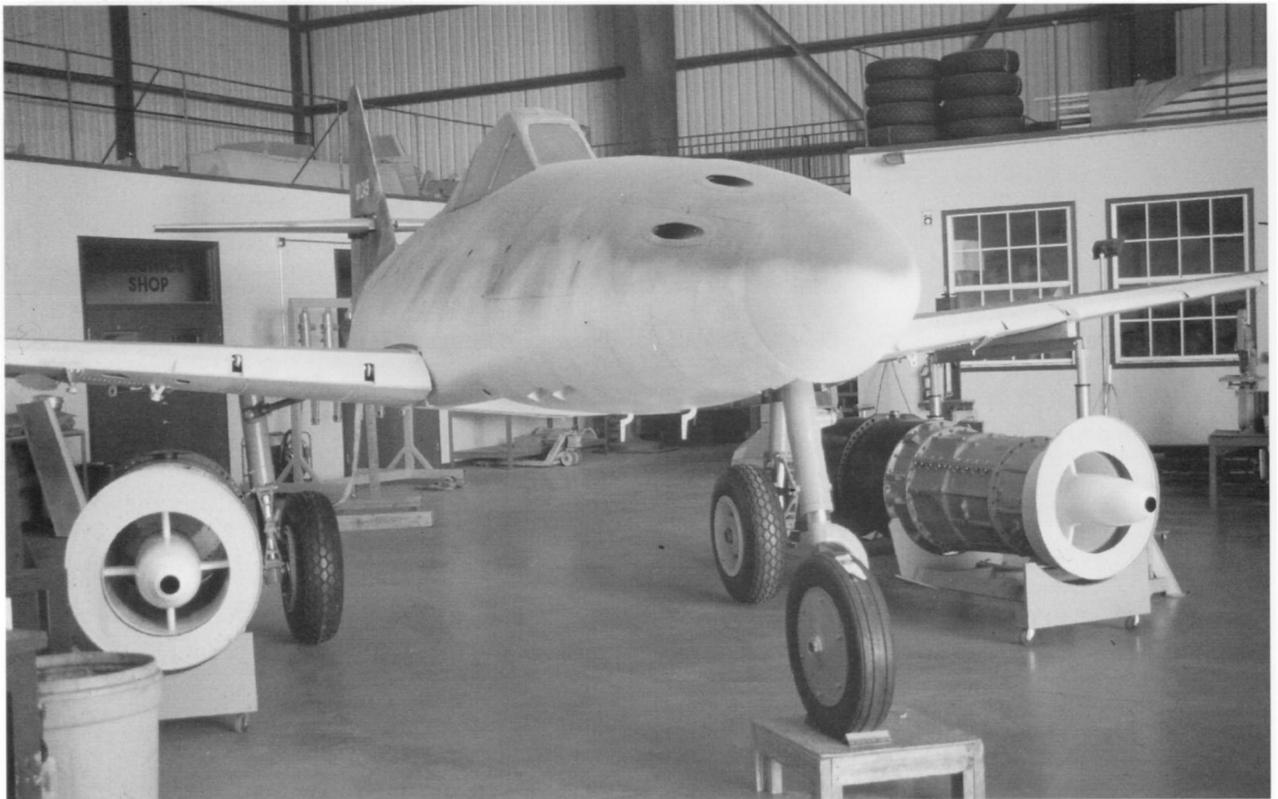
The first replica was due to fly by late 1997 and by March had been test assembled in the hangar. Since the original, and unreliable, engines are not available, modern turbojets are being substituted and these will be fitted into dummies of the originals so that the dimensions remain the same and the engine will look correct even when the panels are removed.
